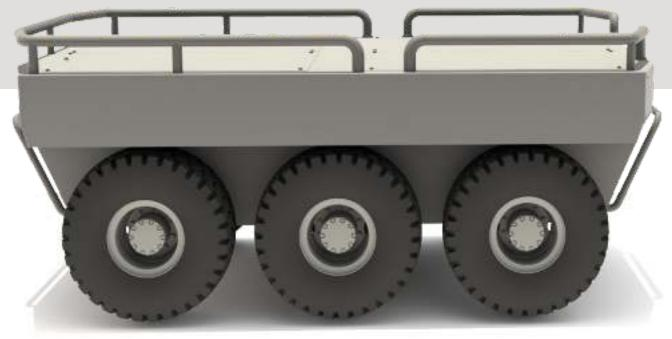
TRAGGER XTV is a high-mobility unmanned ground vehicle (UGV) platform, engineered for full adaptability to challenging terrain conditions. It can operate reliably across all types of surfaces, including mud, snow, sand, rocky, and sloped terrains.
